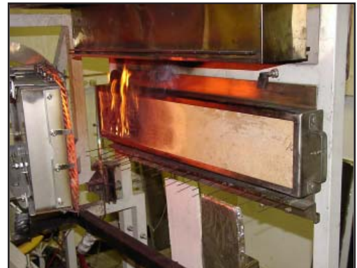
Surface Flammability Test per IMO Part 5
